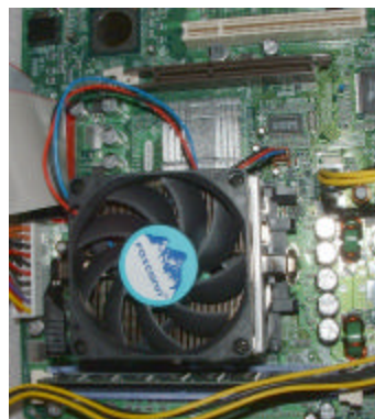
Are all power cables connected? Is the heatsink installed correctly and seated flat on the CPU with thermal compound? Is memory seated correctly?
