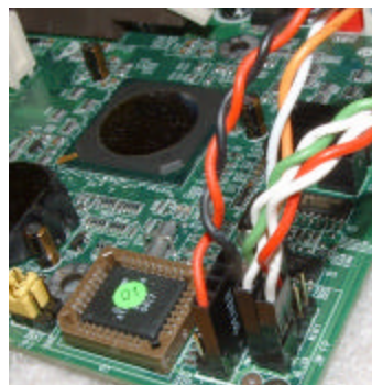
Are the front panel connections on correctly? Try removing the reset button connection if these are separate connections.
