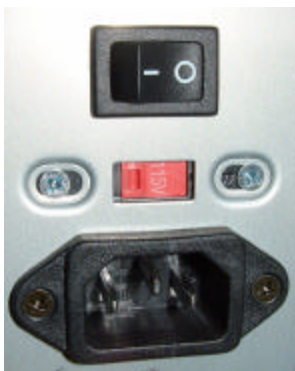
Is it turned on, plugged in, and set to the correct line voltage?
